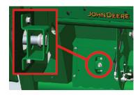
**Critical:** On the 730FD only, the idler belt tensioning bolt should be even with the outside shield.
