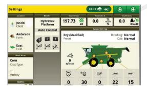
To edit the screen on the extended monitor, it must be brought back down to the Generation 4 display mounted on the CommandARM
