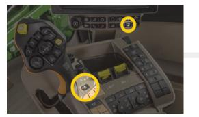
Press the unlock button on the CommandARM or the Control Set-up softkey
