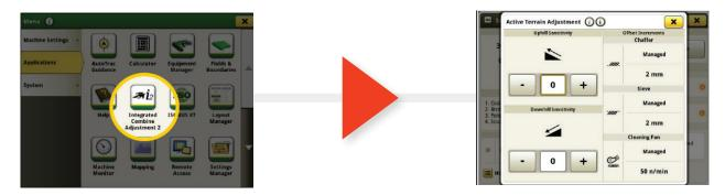
In the Application tab, select Integrated Combine Adjustment 2 2) Adjust sensitivity as needed
