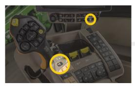
Press the unlock button on the CommandARM or the control set-up softkey. The Controls Set-up page will appear
