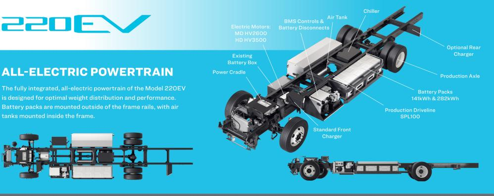
The **power electronics cradle** includes the vehicle's on-board charger, battery disconnect controls, vehicle software, cab heater unit and air compressor. The cradle is located in a single, easily accessible service point, where a traditional diesel engine would be located.
