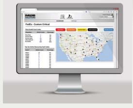
SmartLINQ's web portal provides a geographical view of a fleet's vehicles, color coded by severity. Data can be sorted by diagnostic code, code severity and its geographical location to easily see the vehicle's diagnostics information.
